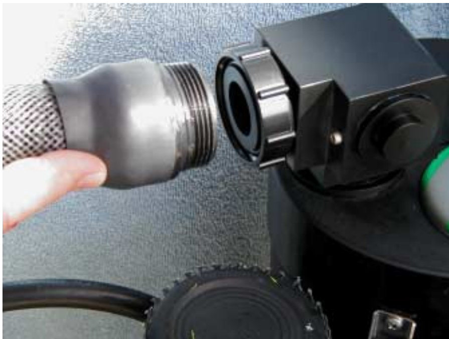
Figure 3 – Attach the breathing hose to the manifold elbow
