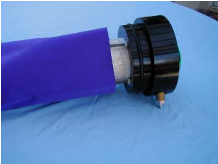
Figure 16 – Counter lung placed over the scrubber
