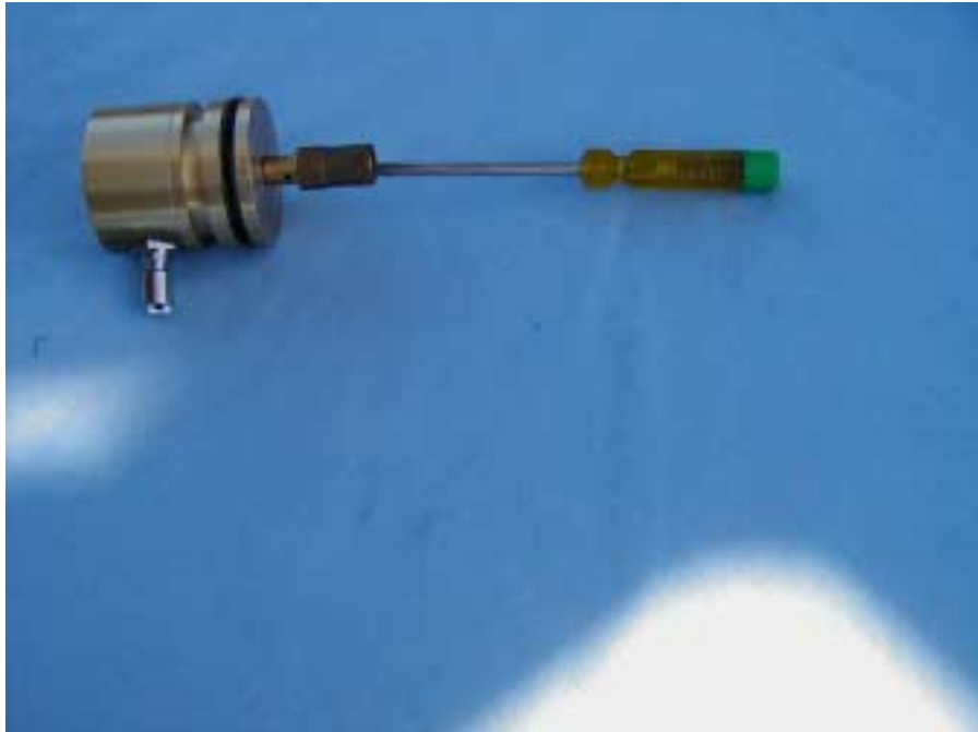
Figure 25 – Valve with screwdriver in place
