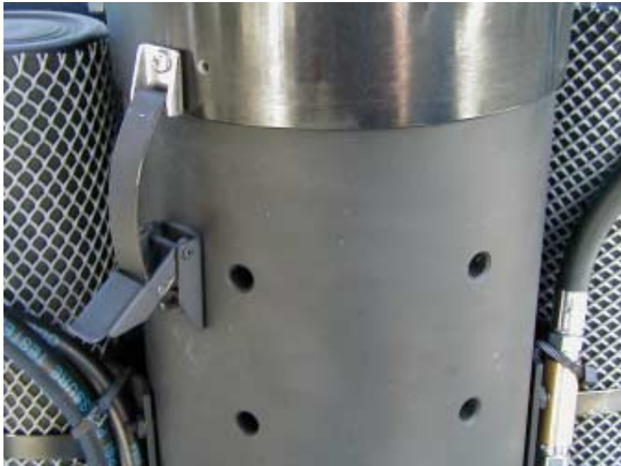
Figure 22 – Line up draw latches and secure
