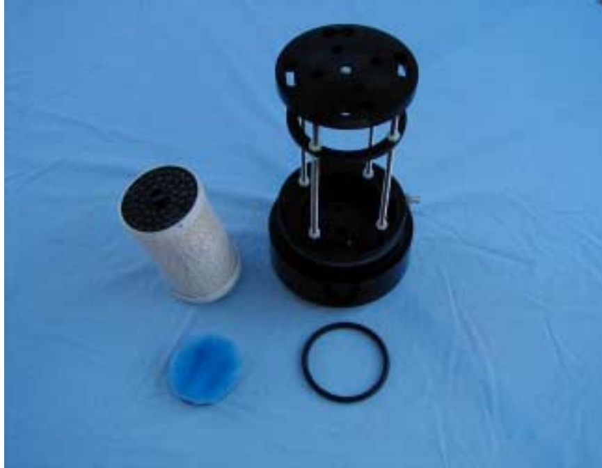
Figure 5 – Scrubber cage, filter pad, scrubber and scrubber O-ring
