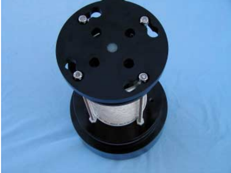
Figure 14 – Bottom plate holding slots
