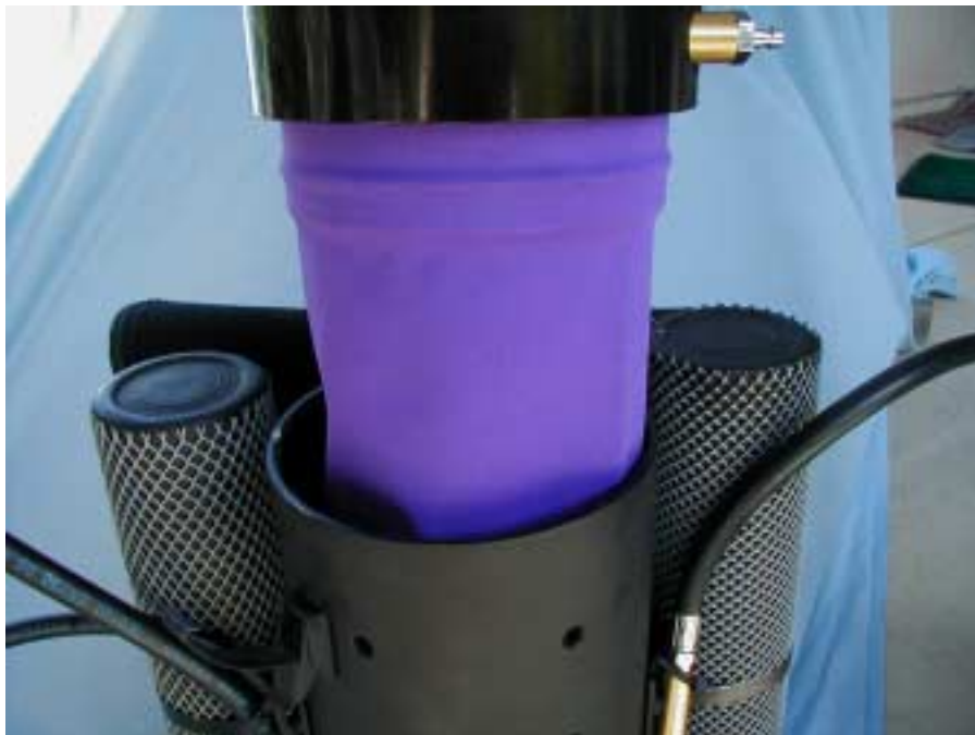
Figure 20 – Insert manifold with counter lung
