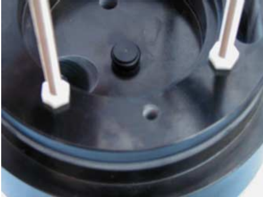
Figure 12 – Inside of the manifold and the dummy plug bottom
