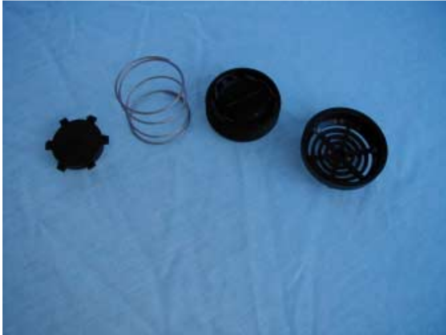
Figure 2 – Relief valve parts
